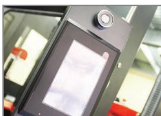
DISPLAY TOUCH GESTIONE REGGIATRICE TOUCH DISPLAY FOR STRAPPING ADJUSTMENT
