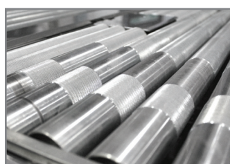
PIANO A RULLI MOTORIZZATI MOTORIZED ROLLER CONVEYOR
